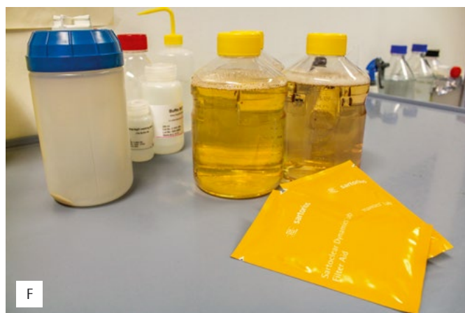
Figure 2: Pouring in and clarification of mammalian cell culture supernatant with 40 g of filter aid using the filter unit Sartolab® RF included in the Sartoclear Dynamics® Lab kit (A – F). A tube is connected to a vacuum pump.
