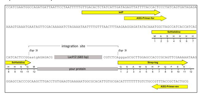
LacP/Z cassette = contains LacZ alpha fragment under control of a separate promoter, which allows alpha complementation of LacZ mutations such as
