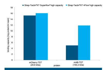
Strep-Tactin®XT 4Flow® high capacity in comparison to Strep-Tactin®XT Superflow® high capacity provides an equal binding capacity for the regular size mCherry-TST, but a 2.5 fold higher binding capacity for the large mAB-TST protein.
